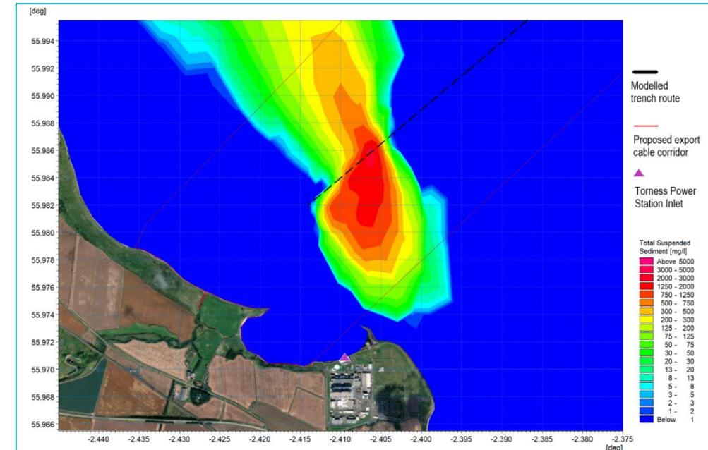
Figure 4: Peak Flood Tide Current 2 Hours Following Cessation of Trenching (High Water - 1 Hour)
