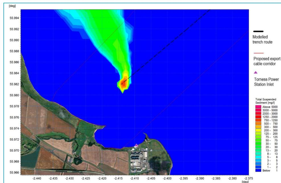
Figure 3: Concluding Stage of Cable Trenching
