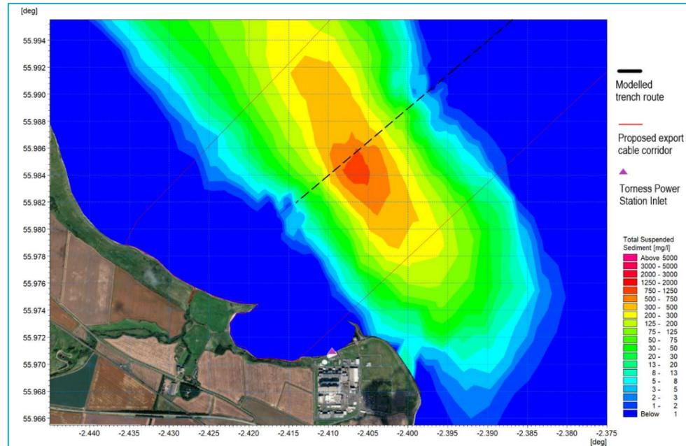
Figure 6: Peak Flood Tide Current 14 Hours Following Cessation of Trenching (High Water - 1 Hour)
