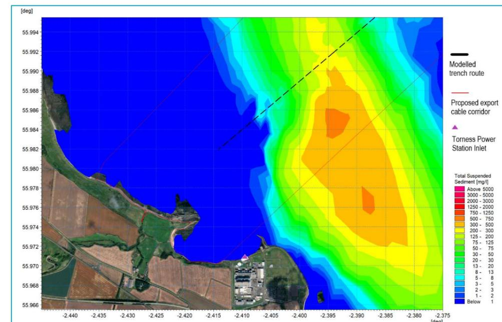
Figure 5: Peak Ebb Tide Current 8 Hours Following Cessation of Trenching (Low Water - 1 Hour)
