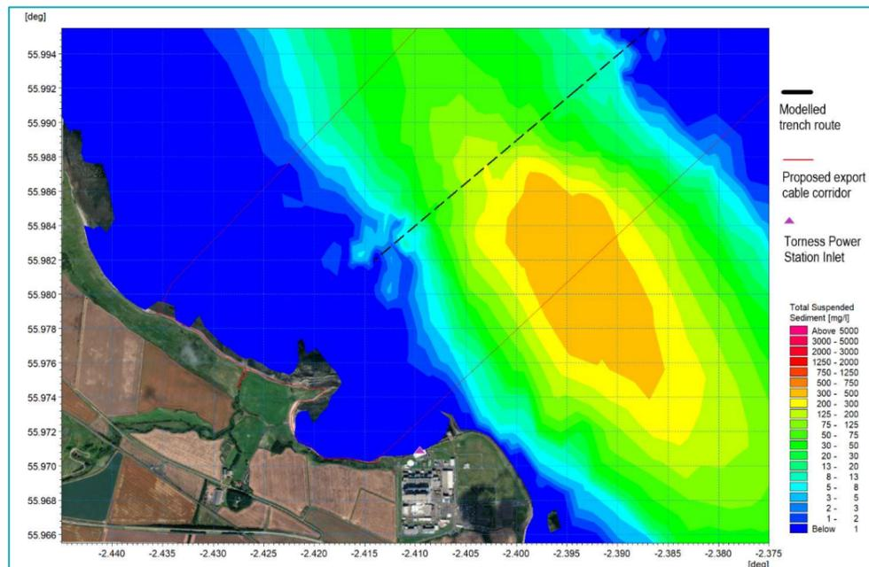
Figure 7: Peak Ebb Tide Current 20 Hours Following Cessation of Trenching (Low Water - 1 Hour)
